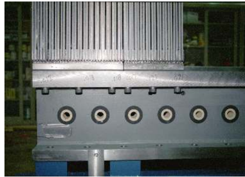
Figure 18. (left) The pneumatic tool used to insert and locate the inner pieces of girder rings for gluing resting on top of a girder ready to have girder rings installed; (right) The outer girder rings following gluing, the black rings are the foam rings used to seal the plastic inserts to the girder surface.
