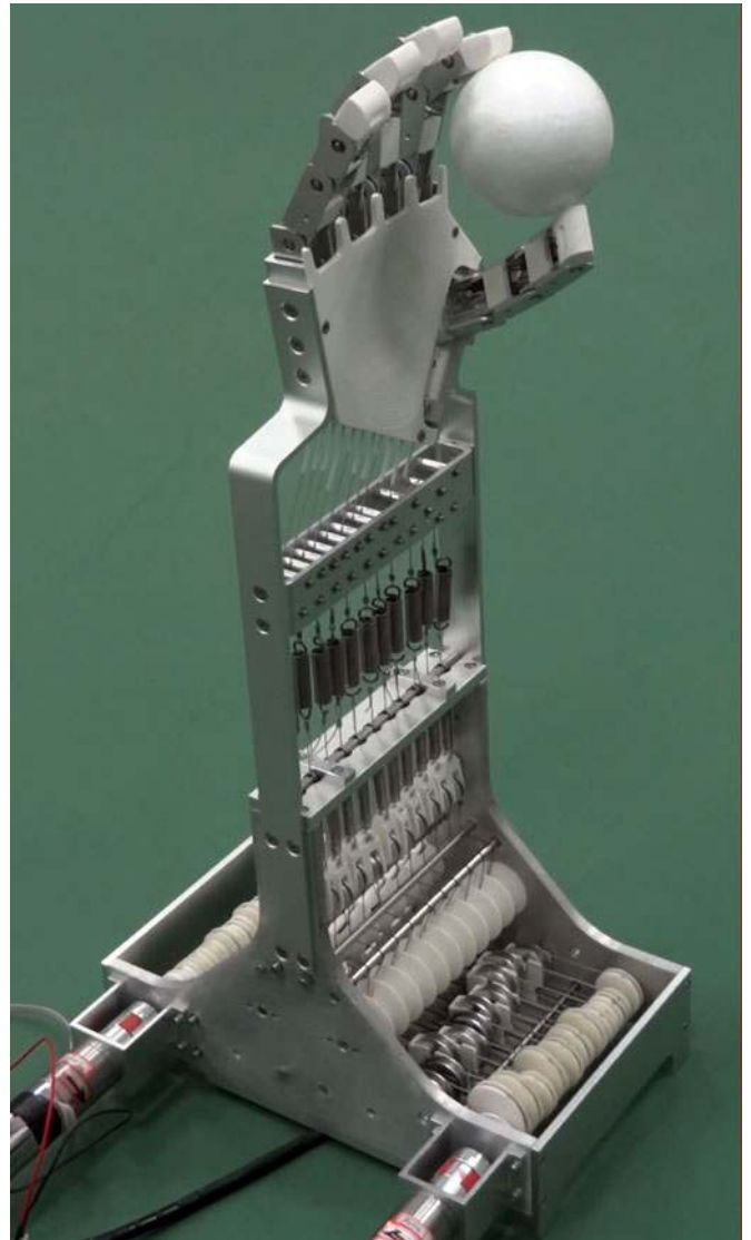
Fig. 1. Prototype of anthropomorphic hand based on the proposed design principle in this paper.
