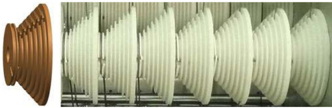
Fig. 12. 3-D solid model of the improved ratio regulator and local view of their assembly on a common axis.
