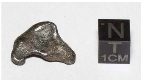
Figure 7: Photograph with a scale marker of the fragment of the Taza meteorite used in the present work.
