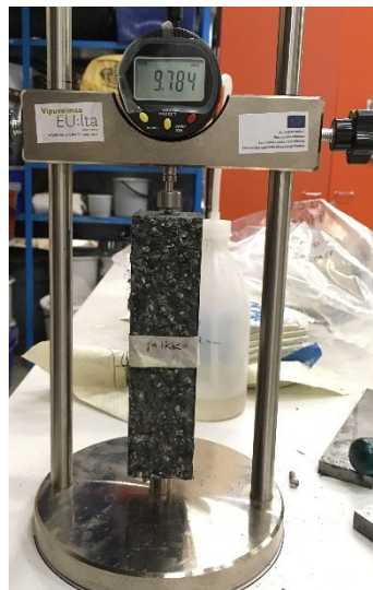
Figure 3: Shrinkage measurement test set up
