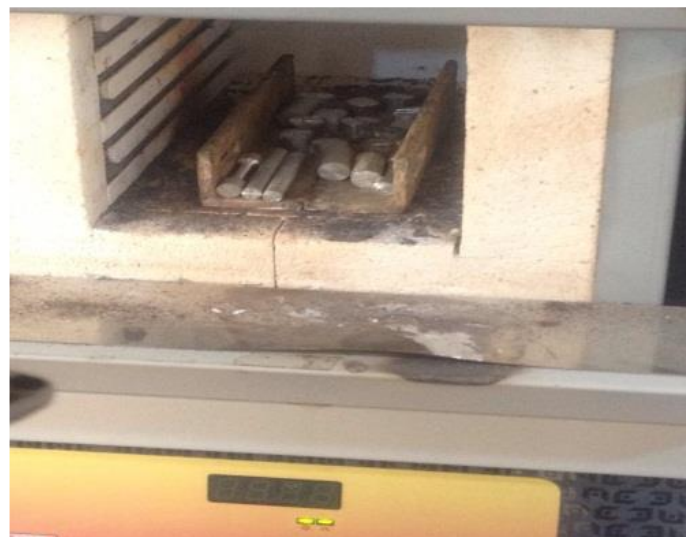
Figure 2. Samples in furnace during heat treatment.
