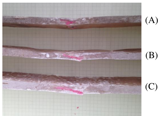
Figure 35: Failure Mode, Side View of (A) Control, (B) 25% ATH, (C) 50% ATH
