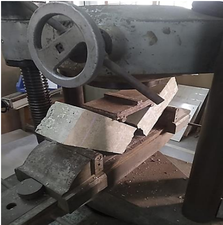
Fig. 6: Flexural strength of beams.
