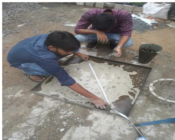
Fig. 1: Slump flow test set up.
