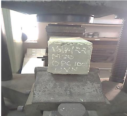
Fig. 5: Split tensile strength of concrete.
