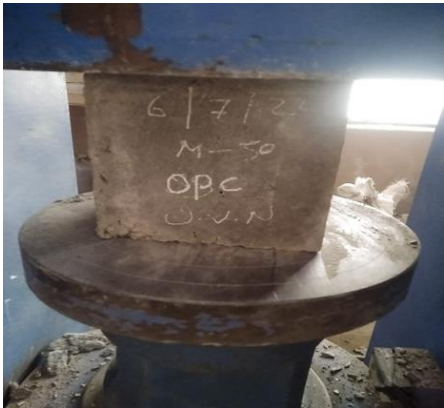
Fig. 4: Compressive test of concrete cube.
