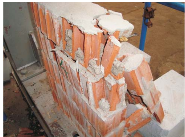
Figure 3. The test sample after failure in compression Slika 3. Ispitni uzorak nakon sloma u tlaku
