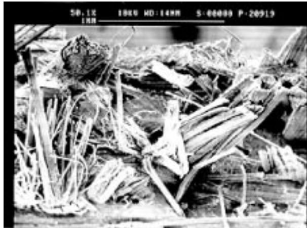
Figure 4. Scanning electron micrograph of fracture surface of PP/flax composite ( V_f = 0.2 and fibre length = 25 mm).
