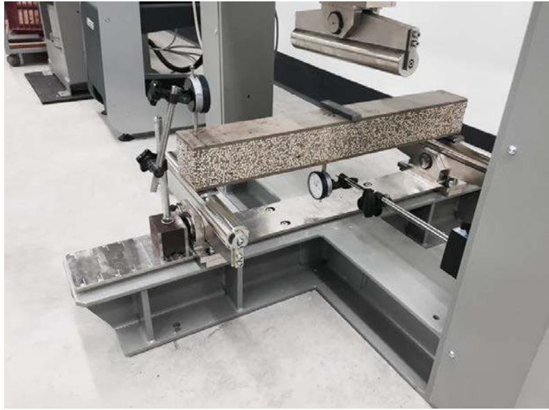
Figure 17: Saturated sample in 3-point loading using Autamax control system and the flexure frame apparatus
