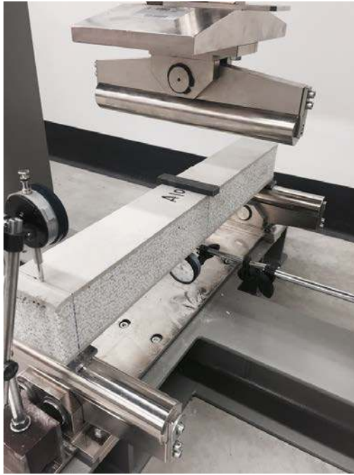
Figure 14: 3-point test in Automax control flexure frame
