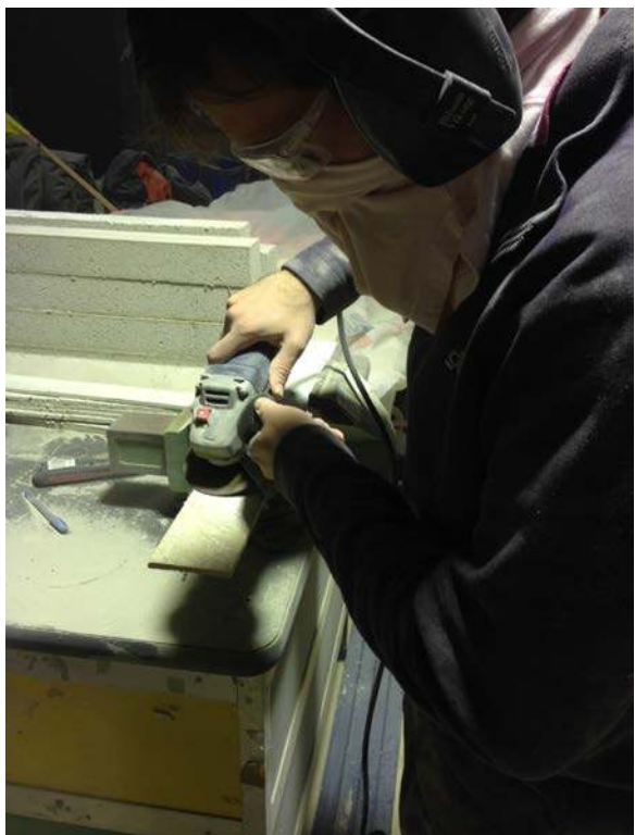
Figure 7: Grinding off the excess core material
