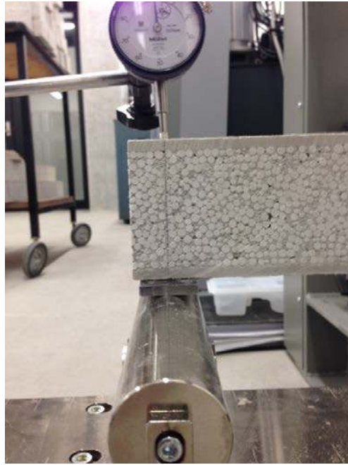
Figure 13: Flat steel between sample and the round support
