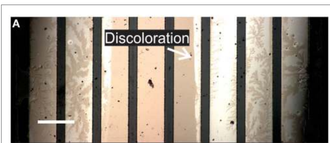
FIGURE 14 | Nomarski differential interference contrast images of fatigue cracks in the top Parylene layer covering three traces of a PAMAP devices after (A) 2k bend cycles and (B) 5k bend cycles. Metal regions are wide, light gray strips and Parylene appears as thin, dark gray strips. The majority of cracks appeared after 5k bend cycles; however, the dashed circle marks cracks present after 2k cycles (circle is 200 \mu\text{m} in diameter).
