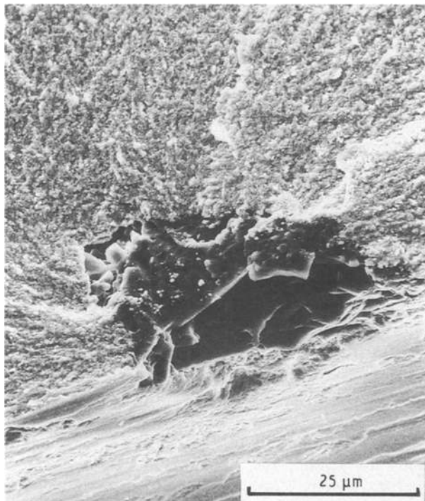
Figure 12 Fracture surface of a ZY5 sample (grain size 0.30 \mu\text{m} ) showing a crack initiating flaw with a size of about 30 \mu\text{m} .
