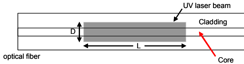
Fig. 2: Optical fiber exposed by UV laser
