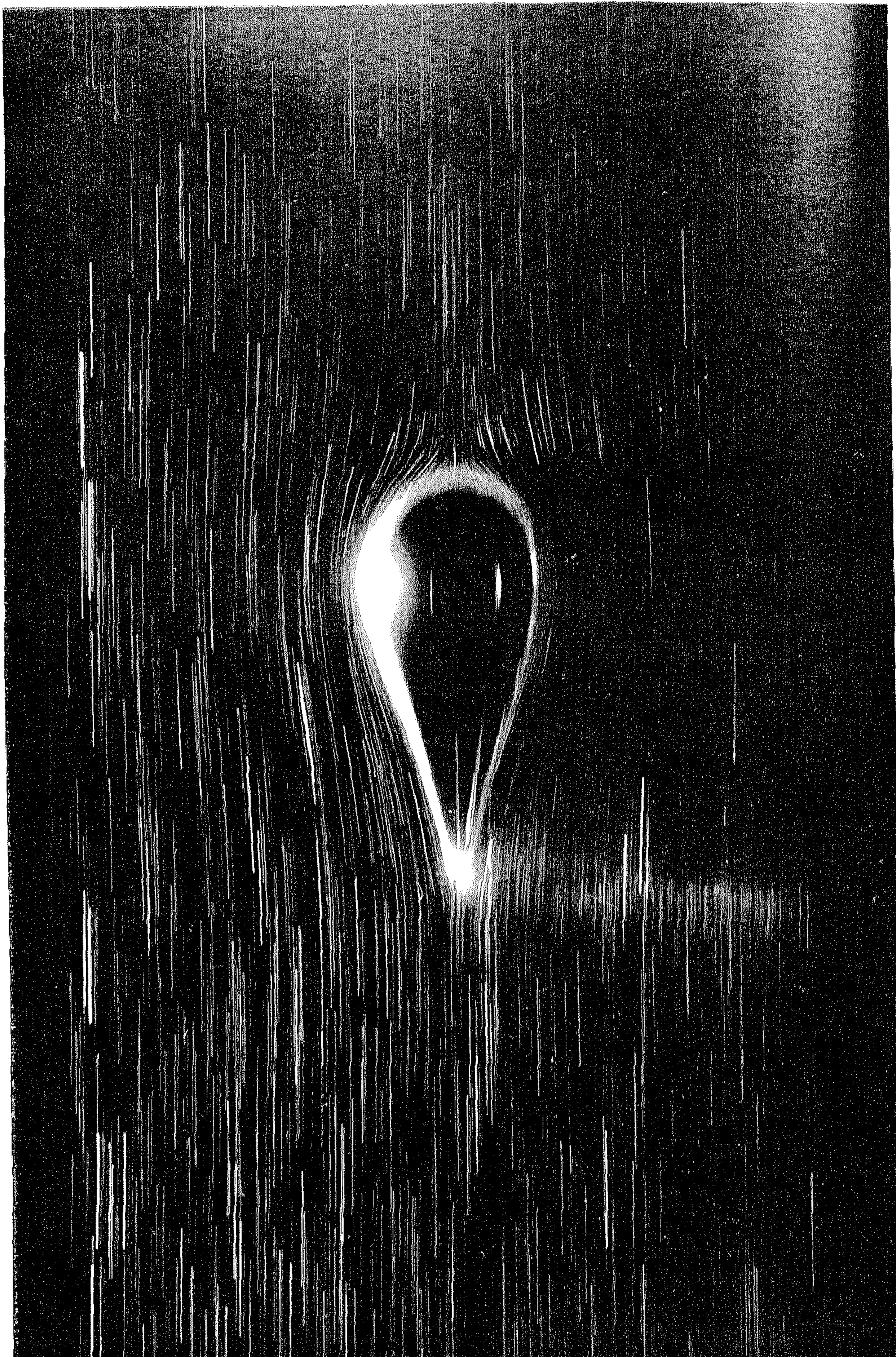
FIGURE 3. Bubble rising in non-Newtonian liquid. \lambda = 0.32 . Bubble volume 13 \times 10^{-6} \text{m}^3 . (Courtesy of Dr P. Thizon.)
