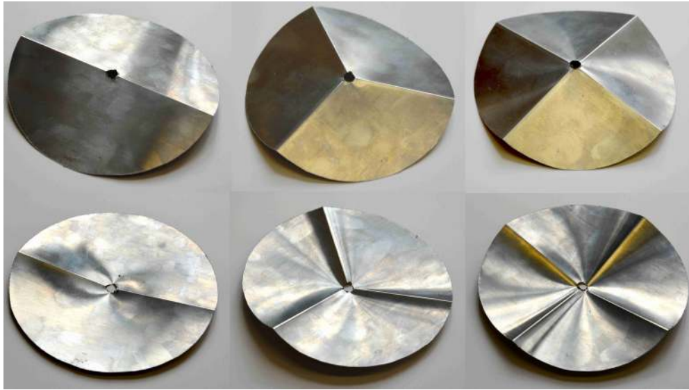
FIG. 1. Disks with 2, 3, and 4 radial creases in the natural (top) and inverted (bottom) configuration.
