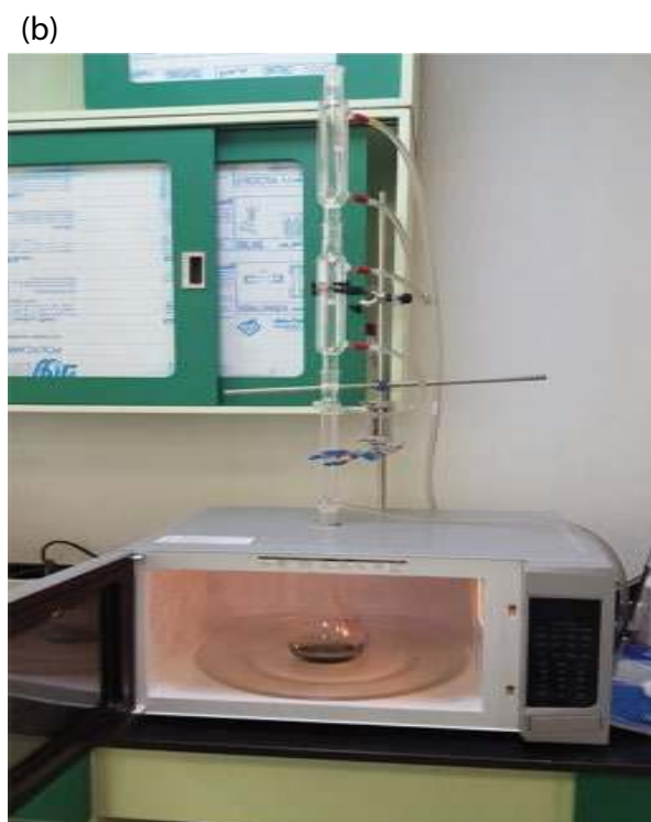
Fig. 1. (a) Schematic illustration of experimental apparatus (1) microwave generator, (2) reaction solution, (3) GO powder, (4) condenser, (5) time display, (6) time adjuster, and (7) power adjuster and (b) picture of the process of degrade the dye inside the microwave system.
