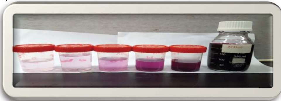
Figs. 2a and b. Picture of MB and arsenazo III dye after degradation at various times.
