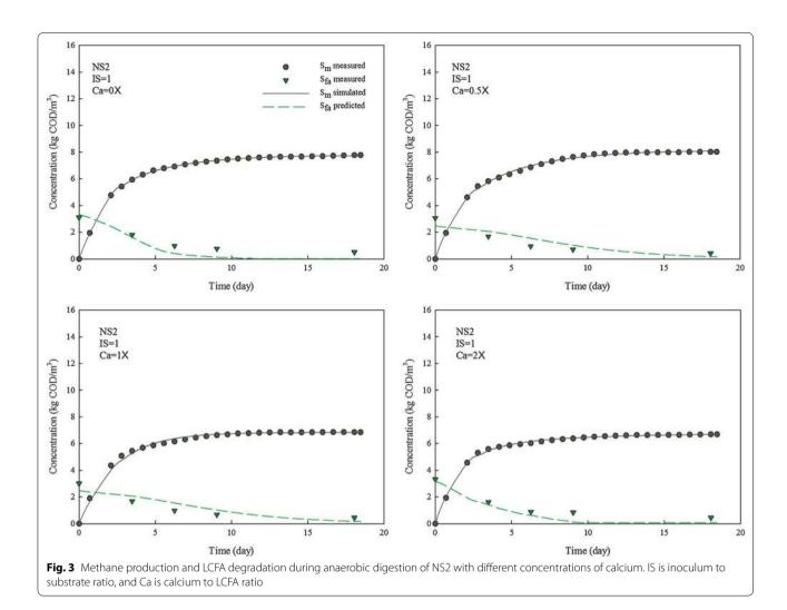
calcium dosing at low I/S ratio while the impacts of calcium ion concentration were less significant at high I/S ratio.
