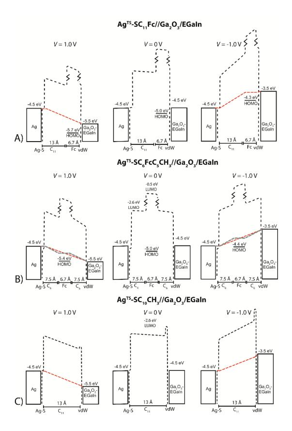
and the HOMO level would be -6.4 eV (if we assume a potential drop of 0.3 eV per 1.0 V applied bias at the SAM// $Ga_2O_3$ /EGaIn interface) and would theoretically participate in the charge transport, as it does at -2.0 V. We do not, however, observe a decrease in the rectification ratio measured at  $\pm$  2.0 V, compared to that measured at  $\pm$  1.0 V.
