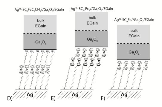
tunneling. Thus, charges encounter a wider tunneling barrier at reverse bias than at forward bias. Since tunneling current decreases exponentially with increasing width of the barrier, a higher current flows at forward bias than at reverse bias, and the junction rectifies.
