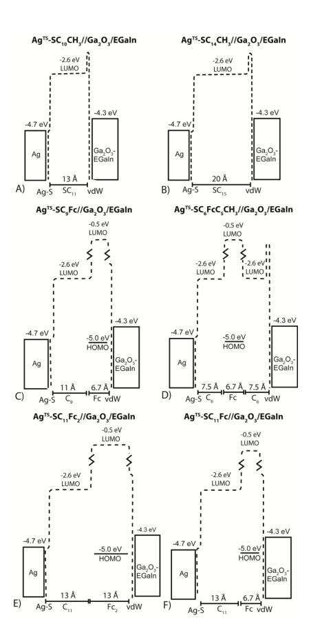
resistance of the layer of  $Ga_2O_3$  is at least four orders of magnitude less than the resistance of a SAM of  $SC_{10}CH_3$  (see Supplemental Information). Furthermore, the high dielectric constant of  $Ga_2O_3$  (~ 10)<sup>70</sup> compared to that of SAMs of alkanethiols  $(2.7)^{71}$  implies that the potential tends to drop along the SAM, rather than the  $Ga_2O_3$ .
