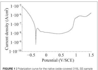
**FIGURE 1** Polarization curve for the native oxide-covered 316L SS sample recorded in  $0.05 \text{ M} \text{ H}_2\text{SO}_4$  in the Ar-filled glove box after initial stabilization at open circuit potential for 30 min (dU/dt = 5 mV/s).
