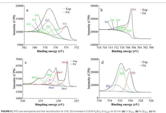
**FIGURE 6** | XPS core level spectra and their reconstruction for 316L SS immersed in 0.05 M H<sub>2</sub>SO<sub>4</sub> at U<sub>OCP</sub> for 30 min: (a) Cr  $2p_{3/2}$ , (b) Fe  $2p_{3/2}$ , (c) Mo  $3d_{5/2-3/2}$ , and (d) O 1s regions (take-off angle: 90°).
