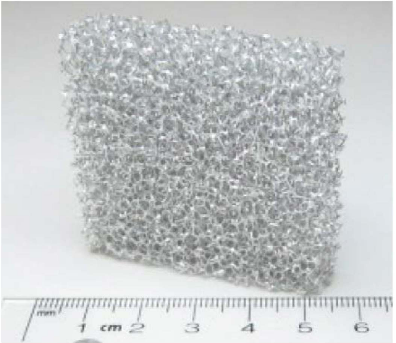
Fig. 19. Aluminum foam sample to mimic cancellous bone. Reprinted with permission from C. Zhang et al. , Measurements of ultrasonic phase velocities and attenuation of slow waves in cellular aluminum foams as cancellous bone-mimicking phantoms, J. Acoust. Soc. Am. , 129(5), 3317-3326, 2011. Copyright 2011, Acoustical Society of America.
