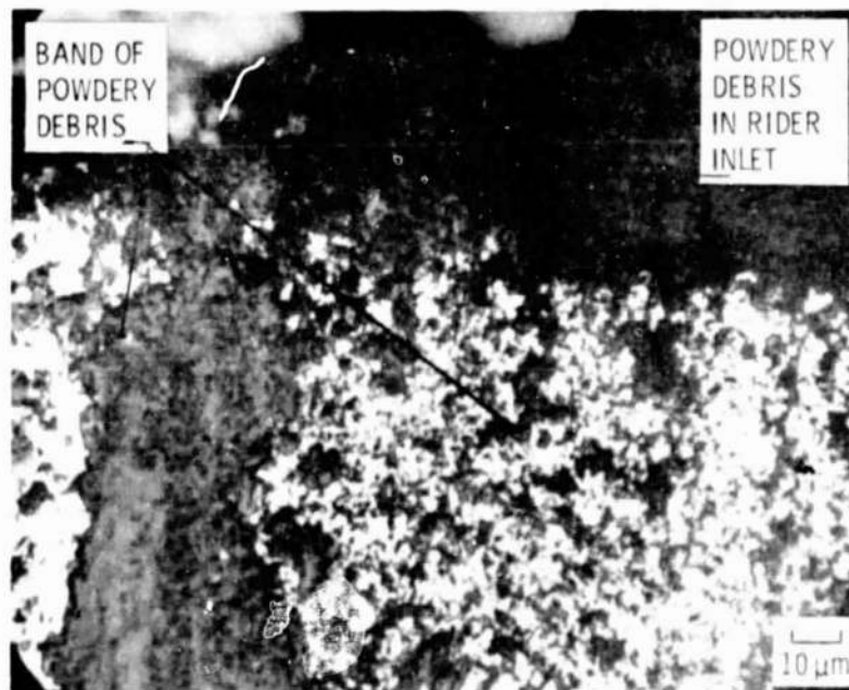
(b) HIGH MAG. VIEW OF POWDERY DEBRIS IN THE RIDER INLET AREA.
