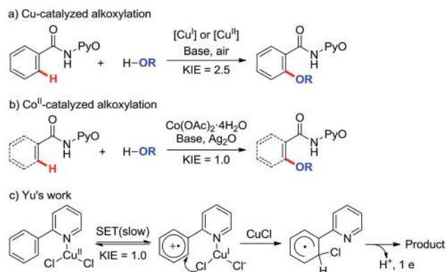
Scheme 1 Copper- and cobalt-catalyzed C(sp 2 )-H functionalization.
