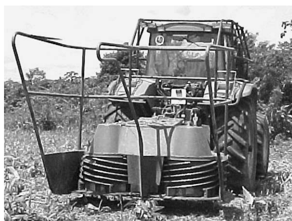
Figure 2. Newly developed bush chopper Tritucap II.
