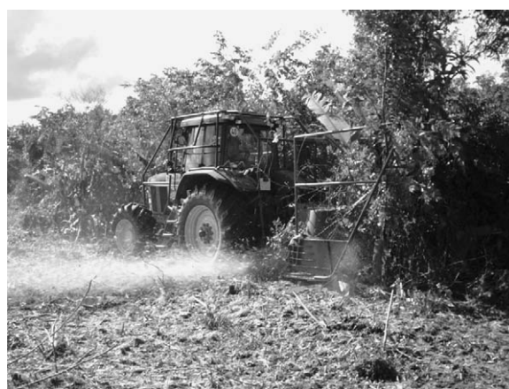
Figure 3. Tritucap II at work in 4-year-old fallow vegetation.
