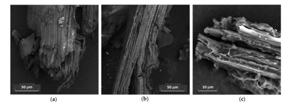
**Figure 8.** FESEM images collected on the as-received wheat-straw biomass before SSRE extrusion ( $\mathbf{a}$ - $\mathbf{c}$ ). FESEM images collected at 15 kV ( $\mathbf{a}$ , $\mathbf{b}$ ) and 5 kV ( $\mathbf{c}$ ) using a BSE detector. Instrumental magnification:  $1500 \times (\mathbf{a}$ , $\mathbf{b}$ ) and  $6000 \times (\mathbf{c})$ .
