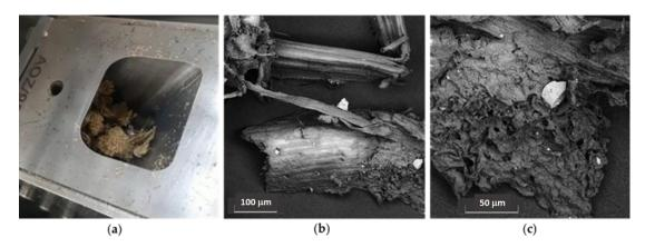
**Figure 9.** Digital image (a) and FESEM images of the wheat-straw biomass soaked with a NaOH solution (10% wt. on dry biomass) overnight at room temperature before (a) and after SSRE extrusion (b,c). FESEM images collected at 5 kV with a BSE detector. Instrumental magnification:  $500 \times$  (b) and  $1500 \times$  (c).
