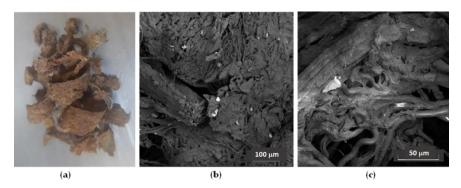
**Figure 11.** Digital image (a) and FESEM images of the wheat-straw biomass that was coextruded with NaOH beads at 190 °C for 1 min at 40 rpm (b,c). FESEM images collected at 5 kV with a BSE detector. Instrumental magnification:  $500 \times (b)$  and  $1500 \times (c)$ .
