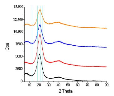
**Figure 3.** XRD patterns of extruded bare PEAA (black line), PEAA with the addition of CPPE (red line), PEAA with the addition of β-CD (blue line), and PEAA with the addition of the β-CD/CPPE complex (10% wt. loading) (orange line) at a temperature gradient of 90/100/110 °C. Cyan lines are eye guidelines to highlight peak positions.
