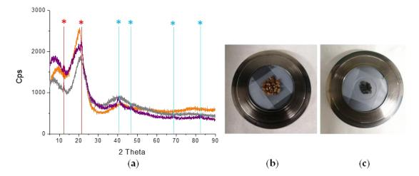
Figure 7. XRD patterns (a) and images of the Pd/ $\beta$ CD-PEAA polymer (Pd/ $\beta$ CD complex 10% wt. loading) mounted on the XRD spinning sample holder before (grey line and (b)) and after reaction (purple line and (c)). The XRD pattern of the bare extruded PEAA is also reported for the sake of comparison (orange line). The catalyst was synthesized using a temperature gradient 90/100/110 °C.
