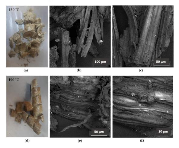
**Figure 10.** Digital images (**a**,**d**) and FESEM images of wheat-straw biomass that underwent soaking with a NaOH solution (10% wt. on dry biomass) overnight at room temperature before SSRE extrusion at 130 °C (**b**,**c**) and 190 °C (**e**,**f**). FESEM images collected at 5 kV with a BSE detector. Instrumental magnification:  $600 \times (\mathbf{b})$ ,  $1500 \times (\mathbf{c},\mathbf{e})$ , and  $6000 \times (\mathbf{f})$ .
