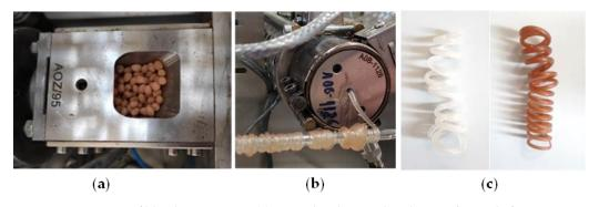
**Figure 2.** Main steps of blend preparation: (a) PEAA beads coated with β-CD/CPPE before extrusion, (b) extrusion of the β-CD/CPPE-PEAA blend, and (c) the obtained blended PEAA: β-CD-PEAA (left) and β-CD/CPPE-PEAA (right) for comparison.
