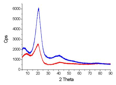
**Figure 1.** XRD patterns of PEAA before (red line) and after (blue line) extrusion at a temperature gradient of 90/100/110 °C.
