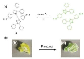
Fig. 12 (a) Mechanism of HABI activation by force or heat (b) HABI was incorporated into poly(urethane), and the materials showed color change after freezing. 104 (b) is adapted with permission from the authors of ref. 104.
