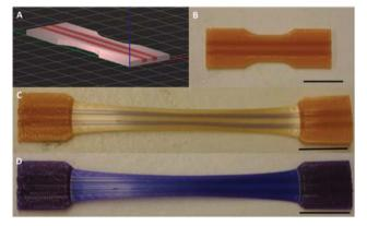
Fig. 17 Preparation of a 3D-printed multicomponent mechanoresponsive sample: (a) CAD representation, (b) Pre-elongation sample, (c) Postelongation sample, (d) Post-elongation sample after 365 nm UV irradiation. Scale bars = 20 nm. 147 Fig. 17 is reprinted with permission from ref. 52, Copyright 2015 American Chemical Society.
