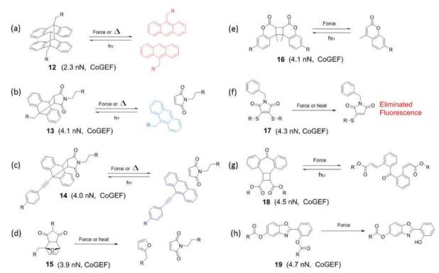
Fig. 5 Structure of various fluorescent mechanophores that are activated by force and display covalent bond scission. (a) Anthracene dimer; (b) Anthracene-maleimide adduct; (c) π-Extended anthracene-maleimide adduct; (d) Furan-maleimide adduct; (e) π-Extended anthracene-maleimide; (g) Methanone-tethered cinnamate dimer. (h) 2-(2'-Hydroxyphenyl)benzoxazole
