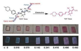
**Fig. 8** Breaking an electrostatic interaction by force resulted in a molecular rearrangement. This rearrangement leads to the release of 3-cyano-4,5,5-trimethyl-5*H*-furan-2-ylidene malononitrile dye; and materials showed a color change, including fluorescent color switching with varying degrees of compressive strain.<sup>73</sup> Adapted with permission from ref. 73, Copyright 2016 Wiley-VCH.
