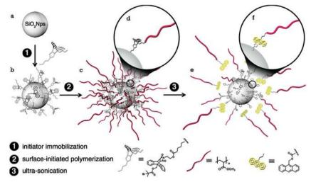
Fig. 23 Illustration of the preparation method of maleimide-anthracene Diels-Alder adduct mechanophore-anchored PMA brush - grafted nanoparticles.<sup>59</sup> Fig. 23 is reprinted with permission from ref. 59, Copyright 2014 American Chemical Society
