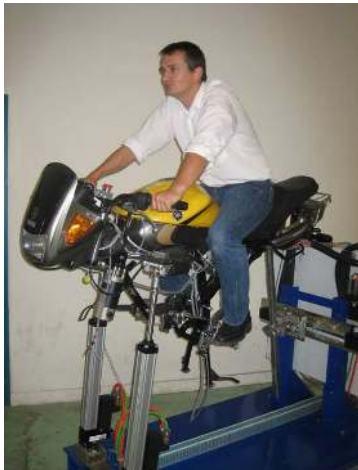
Fig. 15. Constructed riding motorcycle simulator
