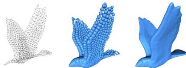
Figure 4: An illustrative example. From left to right: A medial mesh of a bird shape with 400 medial vertices. Reconstruction by the union of the 400 sampled medial spheres. Reconstruction by the union of the enveloping primitives of the medial mesh.
