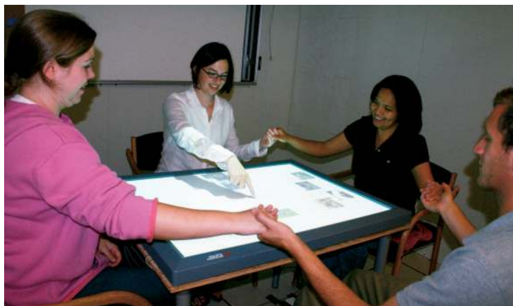
6 Exiting CollabDraw requires a cooperative gesture, to prevent accidental invocation of this potentially disruptive command. To perform the exit gesture, all users hold hands in a chain and the last user touches the tabletop.
