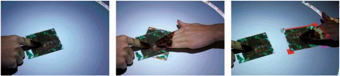
1 The duplicate coordination policy reacts to a whole-element conflict by replicating the contested item.
