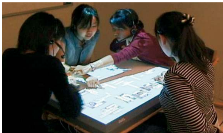
7 Students in one of Stanford University's English as a Second Language courses interact with the MatchingTable, combining English descriptions with photos of their classmates. The one-eared headsets they wear serve several purposes: during some activities, touching words on the tabletop causes them to be pronounced through the earpiece. The earpiece can also provide individually targeted audio feedback regarding the correctness of an action. The microphones on each headset gather speaker-volume data that can optionally be displayed via interaction visualizations.
