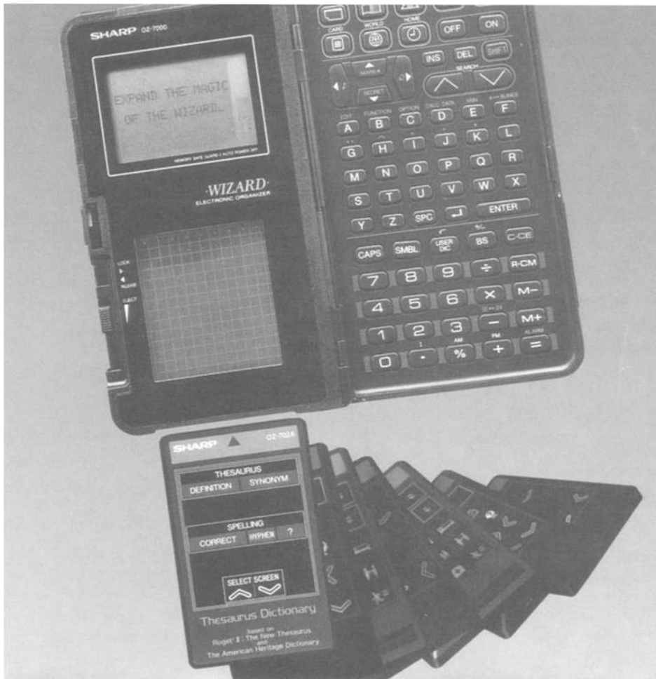
Figure 4. The Sharp Wizard is a compact split case computer with an LCD screen that shows 16 characters on 8 lines. The unit has an innovative memory card slot that offers touch sensitive pads on the face of the card for program control. With its vertical split design, the keyboard is calculator style with special function buttons for internal program control.
