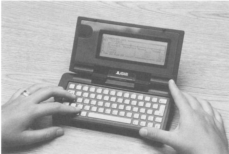
Figure 1. The Atari Portfolio is a handheld MS-DOS compatible computer. In a split case design, the screen is 40 characters by 8 lines on an LCD, and the QWERTY keyboard offers a typing option for user interaction. The computer is an Intel 80C88 running at 4.9 MHz with an MS-DOS 2.11 operating system.
