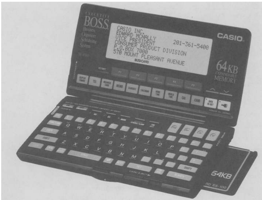
Figure 2. The Casio BOSS (Business Organizer Scheduling System) SF-9500 is Casio's most advanced product in production. It features up to 128K of memory and insertion RAM cards for custom programs. In a split package design, the display is 32 characters by 6 lines, and the keyboard is typewriter style with several additional function buttons on both sides of the case. The display has a tilt-and-lock feature which makes the unit a miniature desktop terminal.
