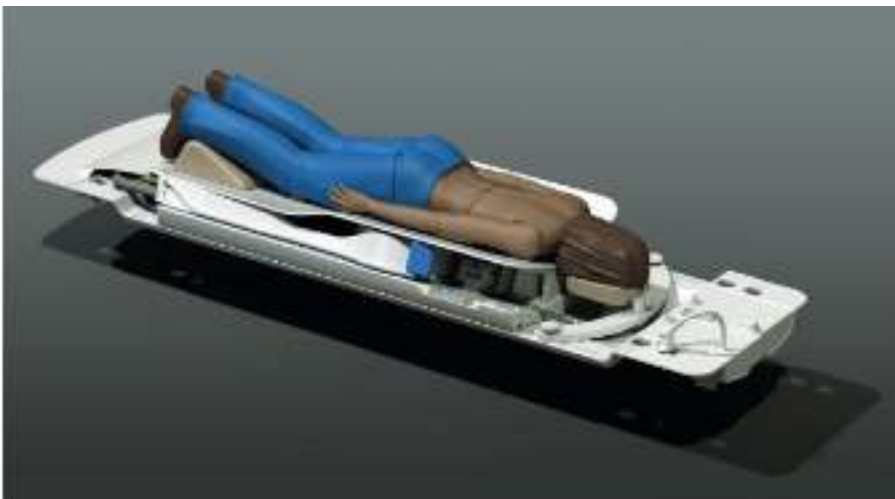
8 Figure 7: Schematic of the HYPMED device. The patient is in a prone position and both breasts can be 9 independently accessed by the two PET rings towards the feet of the patient (from www.hypmed.eu , 10 accessed 16 August 2018)
