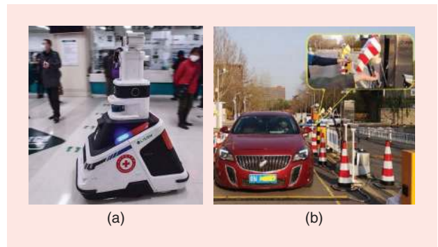
Figure 3. Robots for screening. (a) A robot used for temperature monitoring at a hospital in Shenyang, China. (b) The SHUYU robot developed by Tsinghua University, China, allows for rapid drive-through temperature screening [13].
