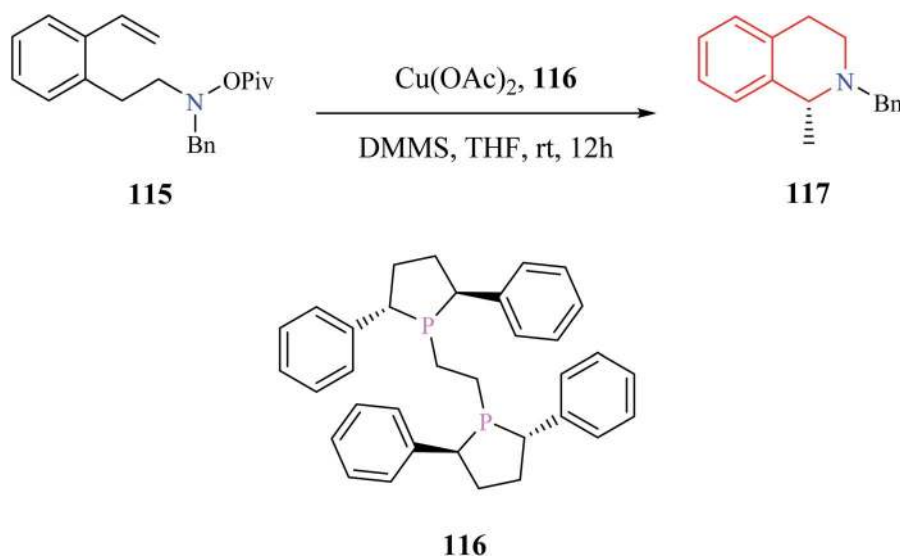
Scheme 22 Enantioselective copper-catalyzed intramolecular hydroamination reaction for the synthesis of compound 117.
