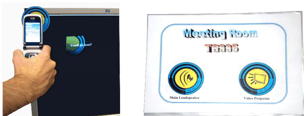
Fig. 7. User selecting a service instance (left), and example service control panel (right).
