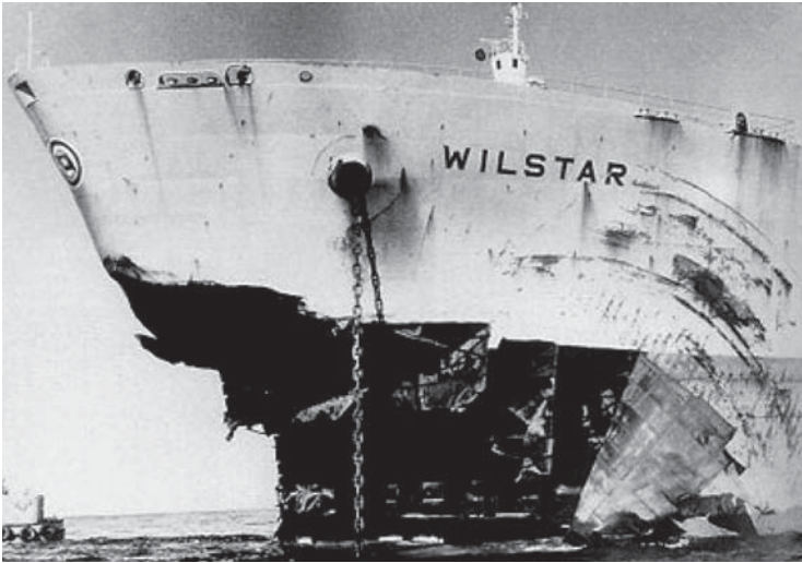
Figure 3. The Wilstar after being hit by a rogue wave in the Agulhas current. To develop standards for the design of ship hulls one must predict not only the likelihood of rogue waves but also the forces that they exert on the hull. Photo credit: DLR.
