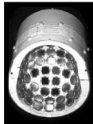
Fig. 5. A view from below of the interior of the helmet electronics of the Neuromag-122, showing the configuration of the 61 dual-channel planar first-order gradiometers (Neuromag Ltd., Helsinki, Finland).
