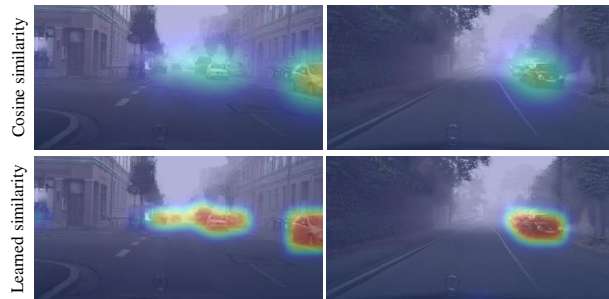
Figure 6. Comparison of attention maps computed using cosine similarity (top-row) and learned similarity based attention (bottom-row). Though cosine similarity based provides reasonable focus on category features, learned similarity obtains more accurate attention.
