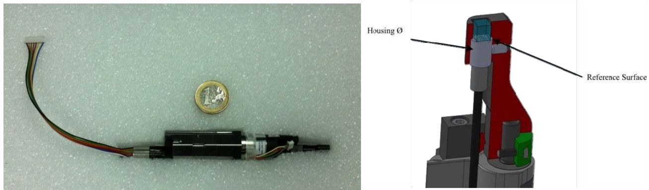
Figure 4. Left: Fiber MOS positioner prototype (December 2011). Right: Positioner button detailed design.
