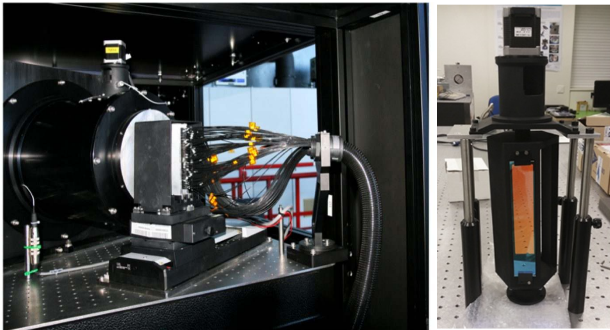
Figure 8: Left: Inside view of the MEGARA optical bench with the two fiber bundles arriving to the entrance focal-plane of the spectrograph. The collimator is also visible in this image with the upper part of the rotating shutter visible in on top of the collimator. Right: View of the rotating shutter at LICA before its integration with the MEGARA collimator.
