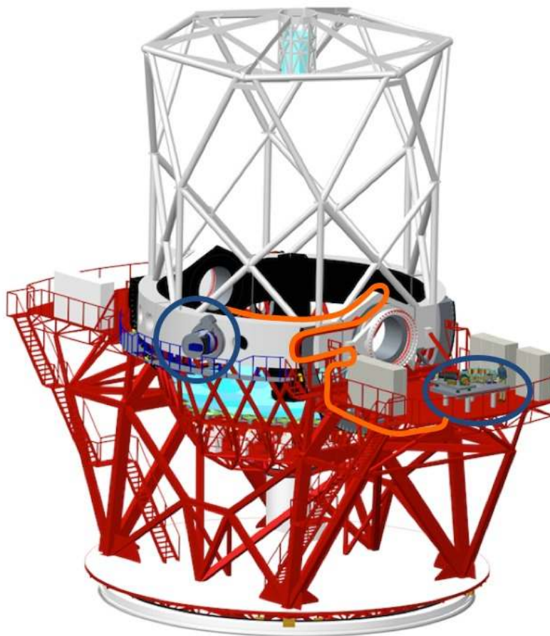
Figure 1: 3D view of the GTC telescope with the MEGARA Fiber-MOS unit placed at its Folded-Cassegrain F focus and the spectrograph sitting on the Nasmyth-A platform (both units encircled in blue). The approximate path of the 44.5m-long fiber link is outlined in orange.
