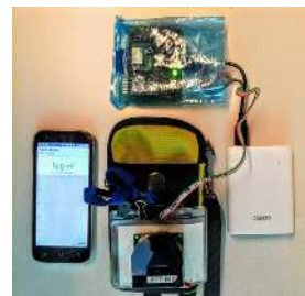
(a) PM 2.5 portable sensor equipped with a GPS, WiFi module and mobile phone connectivity for data logging and visualization [10].
