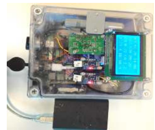
(b) PM 2.5 , gas, and ambient conditions sensor package equipped with microSD memory for data logging and LCD display visualization.
