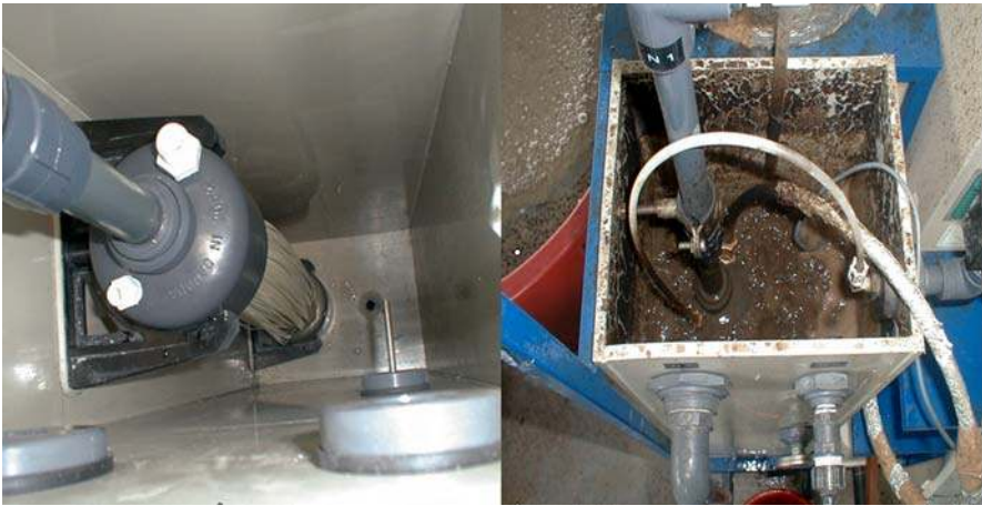
Fig. 4 Hollow-fiber (HF) immersed membrane module (Zenon, Canada) filtrating activated sludge under vacuum
