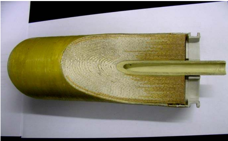
Fig. 5 Spiral-wound membrane part
