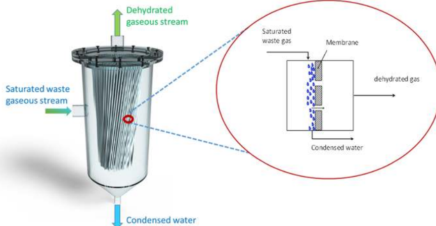
Fig. 1 Scheme of the membrane condenser process for the recovery of evaporated “waste” water from a gaseous stream
