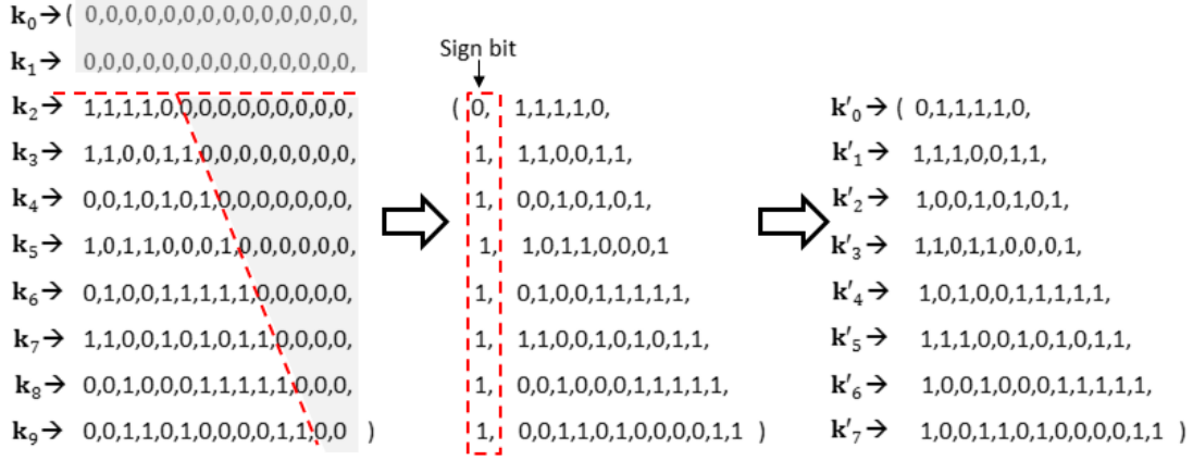
Fig. 2: Optimized probability array by deleting zeros in grey areas, the sign bit indicates the difference between two consecutive block lengths
