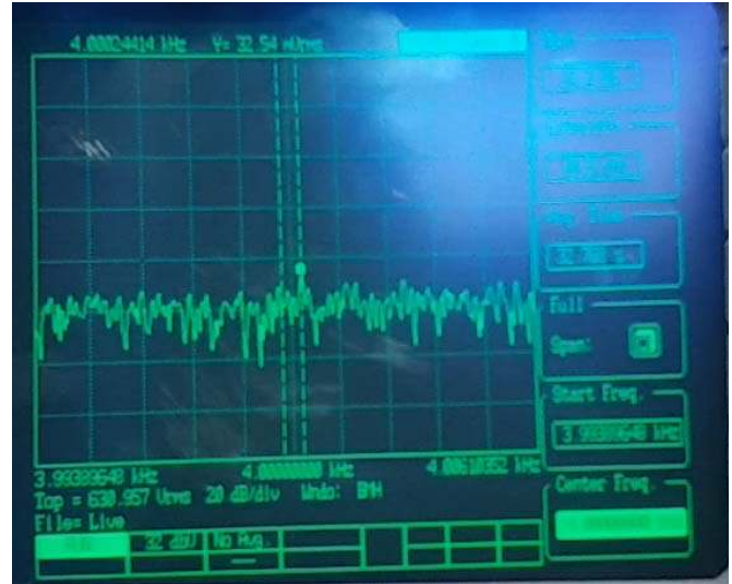
Fig. 18. The noise floor of the system.
