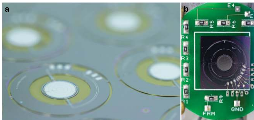
Fig. 6 3D MEMS scan mirror. a Devices on wafer after the release process. b The MEMS scanner after wirebonding to support PCB
