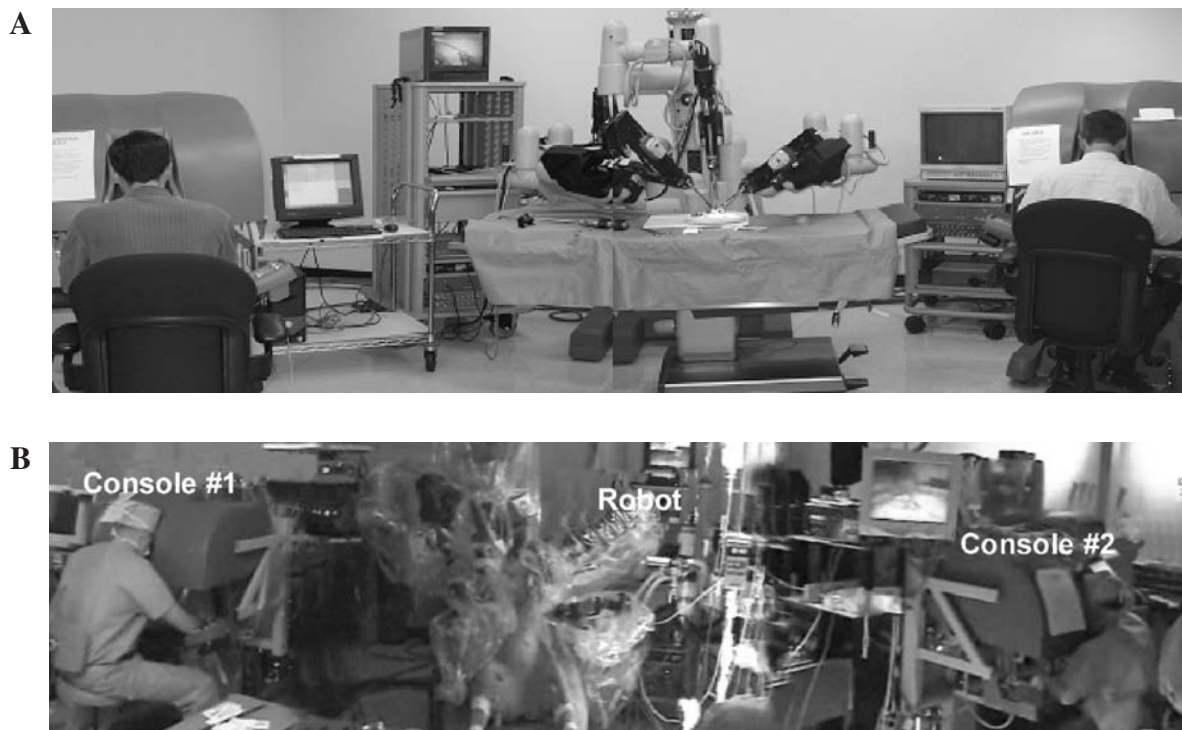
FIG. 2. The da Vinci mentoring system is a novel “two-headed” prototype that uses two standard da Vinci consoles linked together via a special-purpose hardware/software connection. Each unit is fitted with an in-console microphone and speaker system that allows collaborating surgeons and surgeons-in-training to communicate easily with one another. The two consoles can be placed A: side-by-side or B: on opposite sides of the patient.
