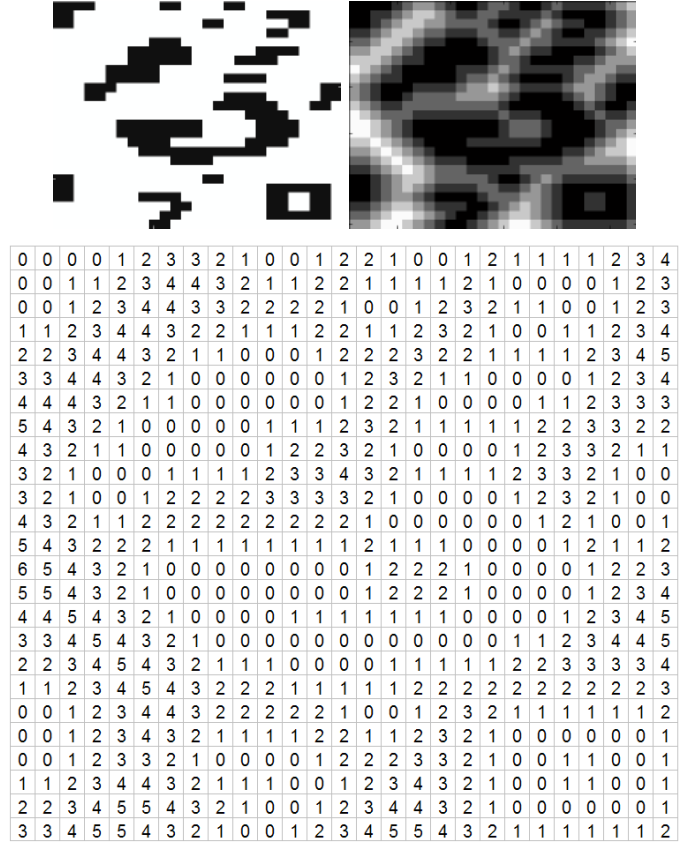
Fig. 1. An example of a distance map that can be used as basis to efficiently compute the similarity between two maps. Given a matrix m with cells marked with a particular value c , here the color black (upper left figure). The distance map d-map (lower center figure) is a matrix containing in every cell the Manhattan distance to the nearest cell with value c in m . A gray-scale illustration of the d-map of m is shown in the upper right figure.
