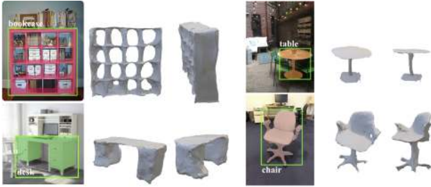
Figure 2. Example predictions from Mesh R-CNN on Pix3D. Using initial voxel predictions allows our outputs to vary in topology; converting these predictions to meshes and refining them allows us to capture fine structures like tabletops and chair legs.
