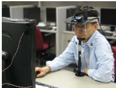
Fig. 2. Our experimental setup for the user study with the ISCAN ETL-500 eye-tracker.
