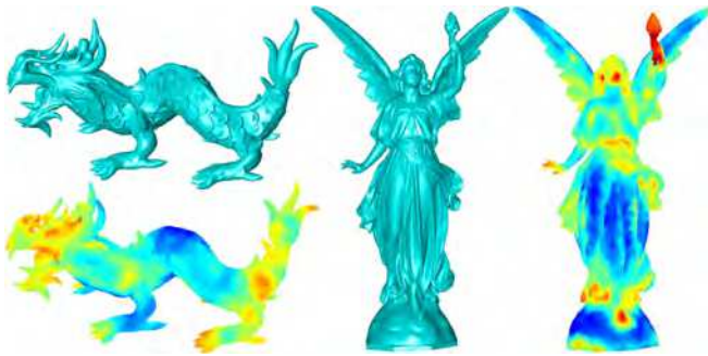
Fig. 19. Saliency detection for meshes containing a large number of vertices. Left: saliency detection for the Dragon model (3.6M vertices); Right: saliency detection for the Lucy model (14M vertices)
