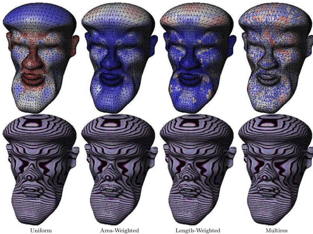
Fig. 18. Head model (7,232 triangles) per-triangle relative scale (top row, white: perfect sampling, red: over-sampled, blue: under-sampled) and with procedural texture applied (bottom row).
